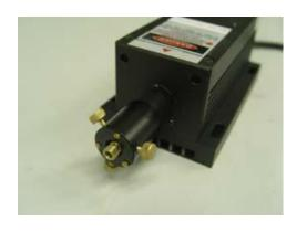
4, Please connect the fiber and the fiber coupler, and adjust the three bolts on the coupler to make the fiber fixed.
